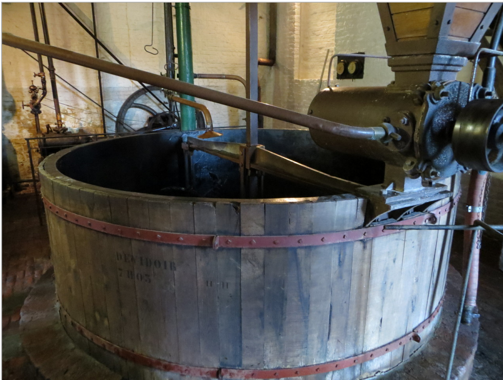
The 19th-century mash tun installed in the Brasserie à Vapeur. Machinery operates on steam power.. Image Credit: Bernt Rostad
